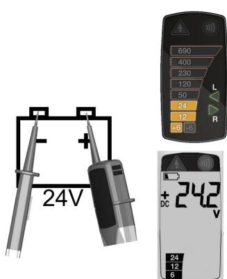
**7.4 AC/DC low voltage measurements**
