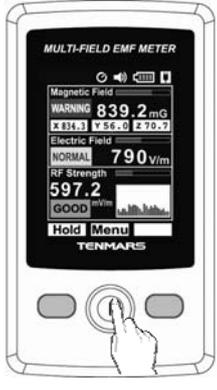
In the measurement mode, press the middle button to enter the main menu
