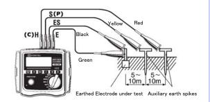
Measurement is more accurate than 3-wire connection by excluding the resistance of E terminal wire.
