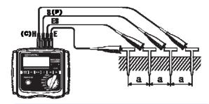
Useful for optimum earthing system design and location, to avoid extra cost of re-working electrode installation. Also for geological and archaeological investigations,
