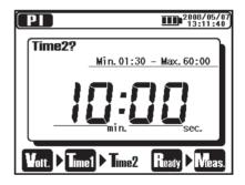
The instrument gets into the Stand-by Mode when settings are made. Setting items for PI measurement are as follows. Refer to the **Setting for Measurement** (=>P.30) and change settings.
