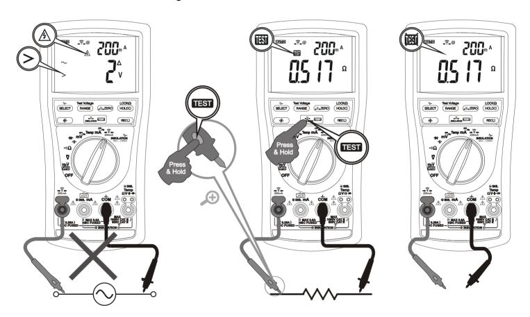
**Lock-Test mode** is recommended for continuous measurements. To apply, press the **LOCK** button momentarily to display the annunciator **LOCK** before pressing the **TEST** button momentarily. The LCD will show both **LOCK** & **TEST** to indicate continuous measurement is active. Press again either button momentarily to release the Lock-Test mode.
